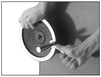
Figure 14. Installing handle on handwheel.
